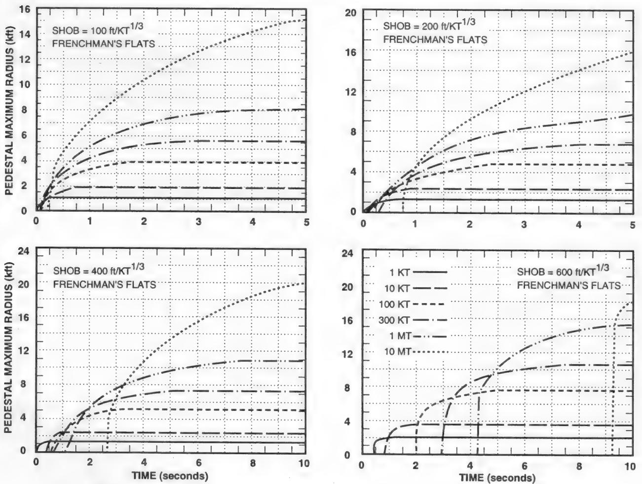
Figure 4.6. Maximum Radius of Pedestal Versus Time for Various SHOBs.
